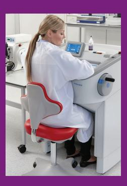
Motorized height adjustment for seated or standing operation (standard for NX70, optional for NX50 models)
